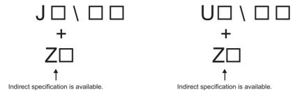
The access destination can be switched with one message, by changing the value of the index register in CPU module programs.
